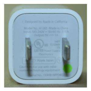
In 2008, Apple recalled the iPhone chargers due to a defect that the AC prongs could fall off the charger and get stuck in an outlet. [15] The faulty chargers had the prongs attached with what was described as little more than glue and "wishful thinking".[15] Apple replaced the chargers with a redesigned model indicated by the green dot marking shown above (which counterfeit chargers inevitably imitate).
