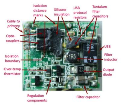
The secondary board contains a standard switching power supply feedback circuit that monitors the output voltage with a TL431 regulator and provides feedback to the controller IC through the optocoupler. A second feedback circuit shuts down the charger for protection if the charger overheats or the output voltage is too high.[11] A ribbon cable provides this feedback to the primary board.
