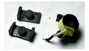
Underneath the next two layers of tape is a 17-turn winding of thin varnished wire, which I think is another shield winding to return stray interference to ground.
