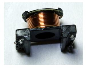
Under the final double layer of tape is the primary input winding, which is 4 layers of approximately 23 turns each. This winding receives the high voltage input. Since the current is very low, the wire can be very thin. Because the primary has about 15 times as
