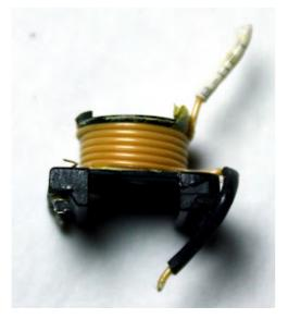
Under the next double layer of tape is the 11-turn heavy gauge primary power winding, that powers the controller IC. Since this winding is on the primary side, it doesn't need to be triple insulated. It's just insulated with a thin layer of varnish.
