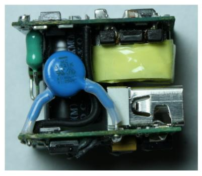
The picture above shows the flyback transformer (yellow) more clearly, above the USB jack. The large blue component is a special "Y" capacitor [4] to reduce interference. The controller IC is visible above the transformer on the top of the primary board. [5]
