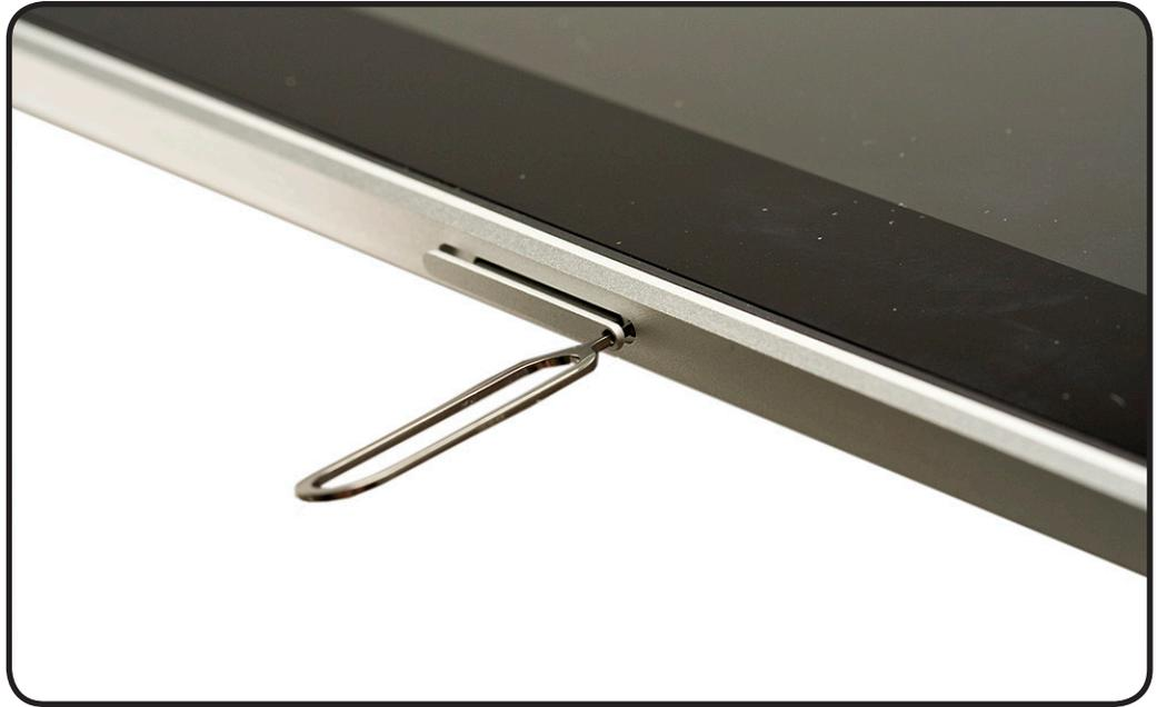
2. Press firmly and push the tool straight in until the tray pops out. (If you don't have a SIM eject tool, you can use the end of a paper clip.)
