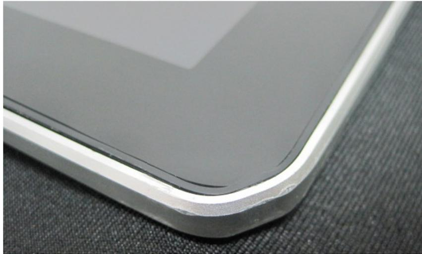
Corner dent resulting in multiple cracks:
