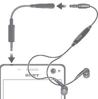
• Plug the headset connector into the Mobile TV antenna cable.
