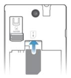
Remove the battery cover, then insert the SIM card into its slot with the goldcolored contacts facing down.
