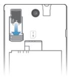
Remove the battery cover and insert the memory card with the gold-colored contacts facing down.
